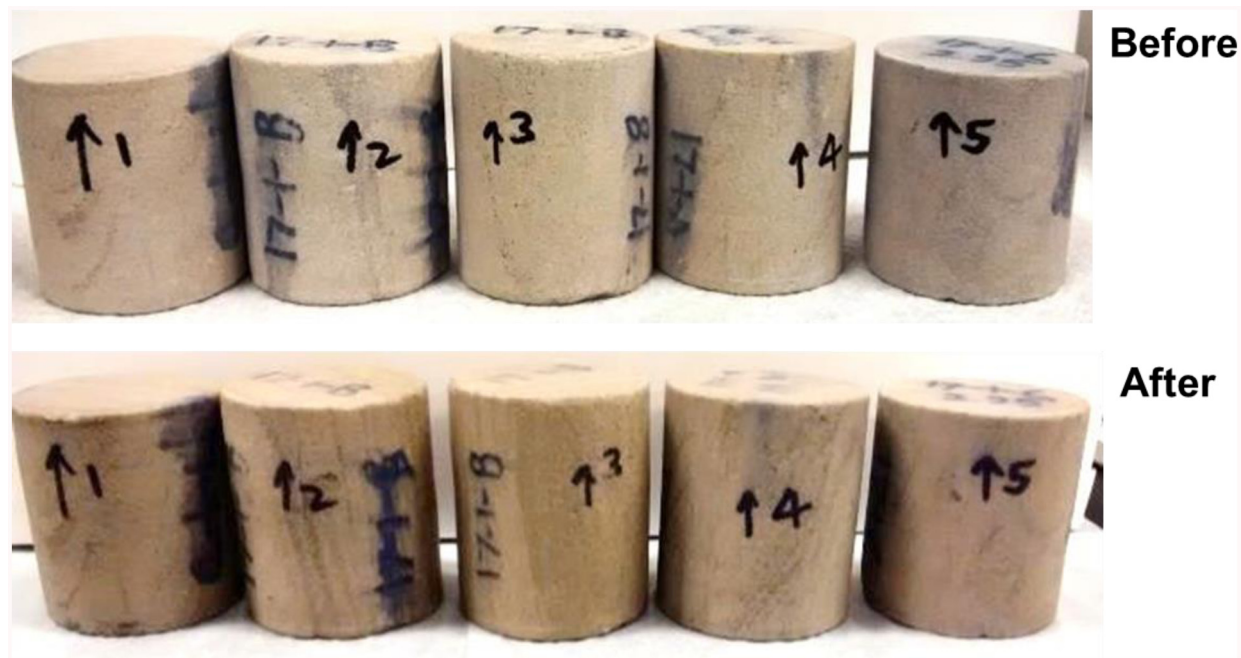
Figure 19—The reservoir coreplugs before and after completion of the coreflood.
