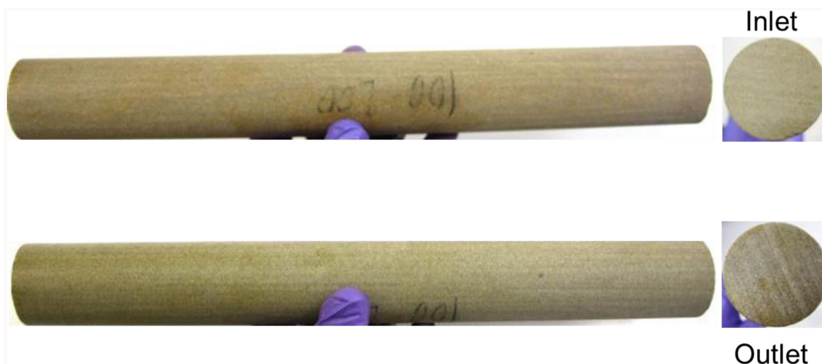
Figure 13—The Berea core after completion of the coreflood. No streaks of unswept oil were observed upon visual inspection.
