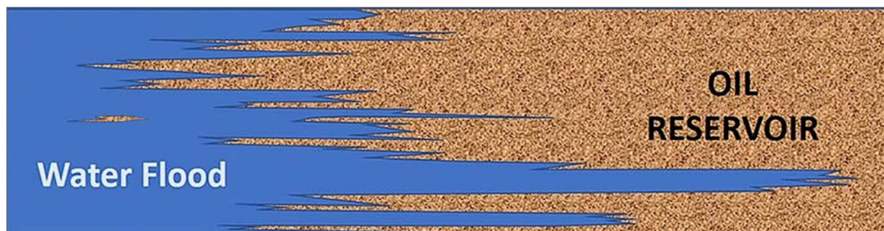
Figure 2. Diagrammatic representation of viscous fingering seen when low-viscosity water (blue) displacing higher viscosity oil (brown). Flow is from left to right.
